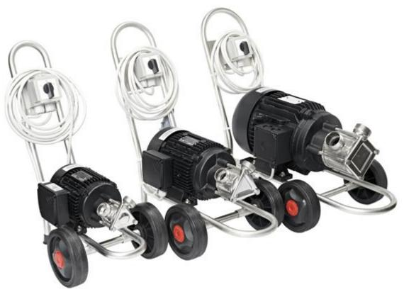
Flow rate up to 600 lt/min Head up to 25 mt Operating temperature max 70°C Operating pressure max 3 bar Motors from 0.4 HP to 6 HP - 700/900/1400 RPM AISI 304 high thickness stainless steel pump casing and synthetic rubber impeller Suitable for viscous liquids with suspended solids
